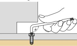
If an object below the long handle is interfering, the end of the long handle can be gripped to make operation easier.
