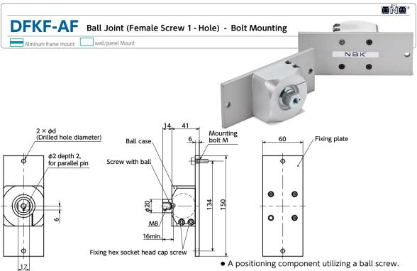
Material/Finish **RoHS** DFKF-AF A6063 Ball Case Anodized S45C Screw with ball Trivalent Chromate Treatment Fixing Hex Socket Head Cap Screw SCM435 (M5×16mm) Ferrosoferric Oxide Film SS400 Fixing plate
