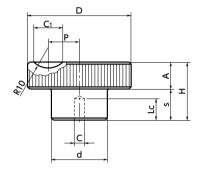
HAK-R With reamer bore and grip mounting hole
