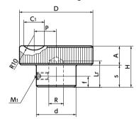
HAK With pilot hole and grip mounting hole HAK-N With pilot hole and without grip mounting hole
