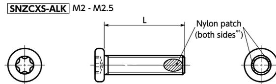
\*1: For dimension L of under 4 mm, nylon adhesion is on one side.
