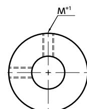
\*1: In a case where the bore diameter is  $\phi$  4 or less, the set screw is used in only one place.
