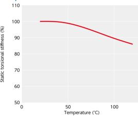
This is a value under the condition where the static torsional stiffness at 20℃ is 100%.
