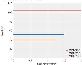
These are initial slippage load values of hubs and a spacer.
