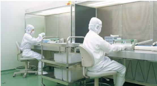
Cleanroom Packing Cleanliness Level In a cleanroom: ISO Class 6 (Class 500*1) Clean bench: ISO Class 4 (Class 10*1)
