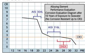
Pitting Corrosion and Crevice Corrosion Countermeasures PRE value (Pitting Resistance Equivalent) PRE=%Cr+3.3×%Mo+16×%N;
