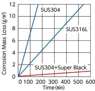
This graph compares corrosion weight loss of a test piece in 6% ferric chloride solution over time. Comparing over the same time period, the mass loss due to corrosion of super black is much less than that of SUS304 and SUS316L, which confirms the good corrosion resistance of super black.
